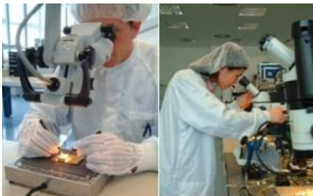
Receiver assembly (left) and fibre-chip coupling (right)
