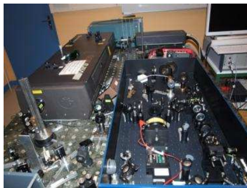
Fig. 8 : Photograph of the 800 nm teraHertz time-domain spectroscopy setup.
